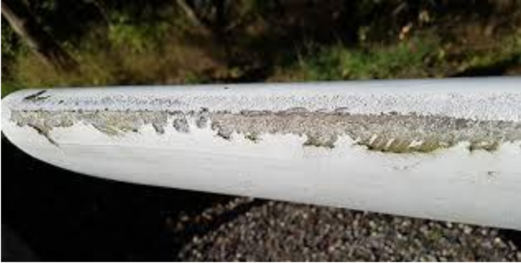
Wind turbine blade with damage on the leading edge Courtesy of Jakob Ilsted Bech
