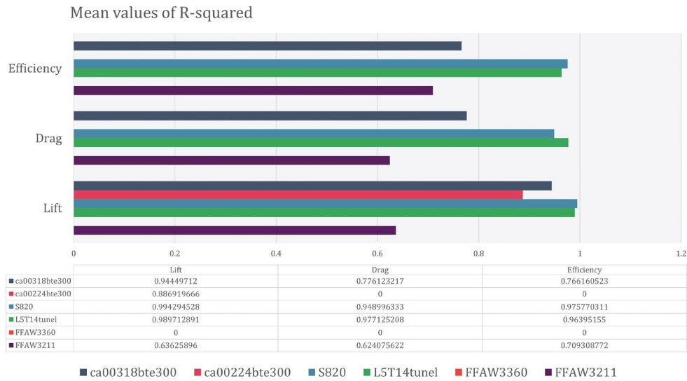
Figure 49 Mean values of the R-squared metric for airfoils not considered in the dataset.
