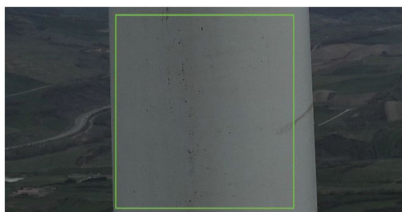
a) Pitting located at the leading edge of blade A. Damage located at the 68% of the span.
